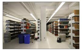
There is also static cantilever shelving installed in the off-site storage facility on the first and second floor. Though mobile was used on the lower level, only static could be installed on the higher floors due to load capacity. End panels were omitted altogether to save on costs—again, since this is a private facility.
