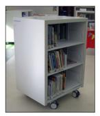
In the children's area, cantilever shelving was outfitted with a custom base, wrapped in solid surface and then placed on heavy-duty casters so that the area is completely reconfigurable on the fly by the library staff.
