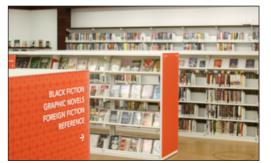
Special red, acrylic end panels were used on the cantilever-shelving units in the showcase space on the main level of the library called The Center for the Reader.
